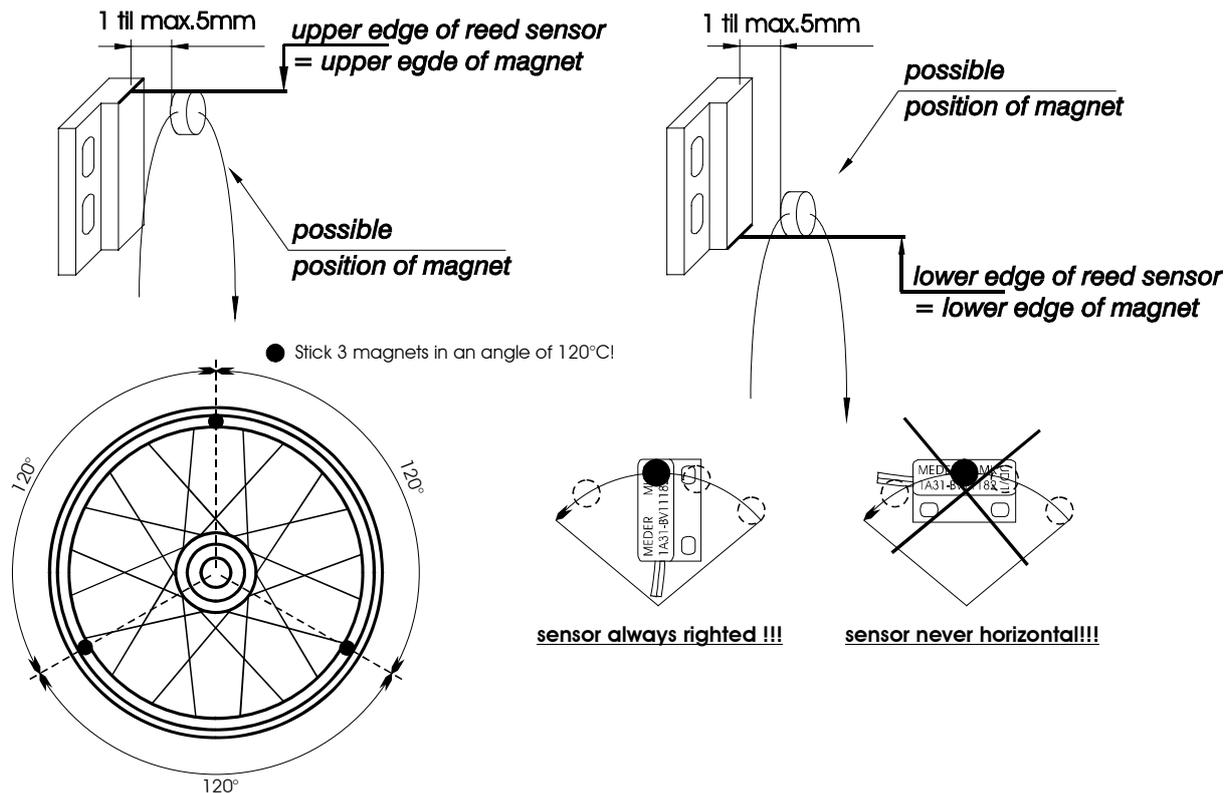
Install the sensor and the magnets according to the sketch. The mentioned dimensions refer to the reed sensor of NOVA-MMB.
